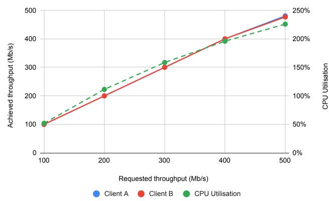
Echo servers with extra work Equal priorities, Separate cores. Round robin TX MUX
